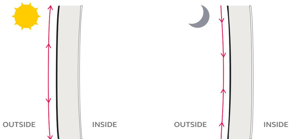
If the hooks on the multipoint lock are not thrown throughout the day and the centre keep setting is too tight, the top and bottom of the door will be in unsupported tension and will eventually stand proud of the inner face of the profile. This will make the hooks on the lock to become stiff, as they cannot draw themselves into the hook keep.
